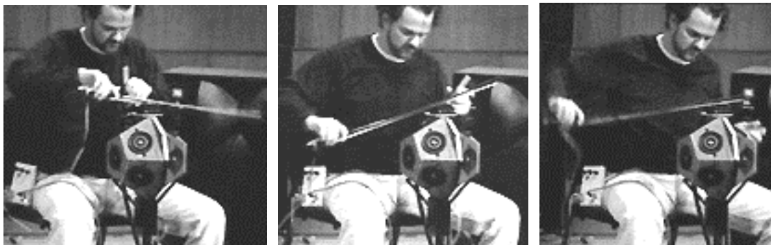
Figure 8. Three frames from a performance of the Lobster Quadrille . Note how the Fangerbored, which is used to "play" the comb filters, is rotated to different positions.
