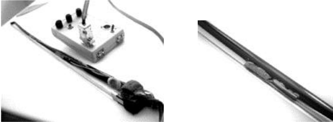
Figure 3. (a) R-Bow, and (b) FSR on R-Bow.
