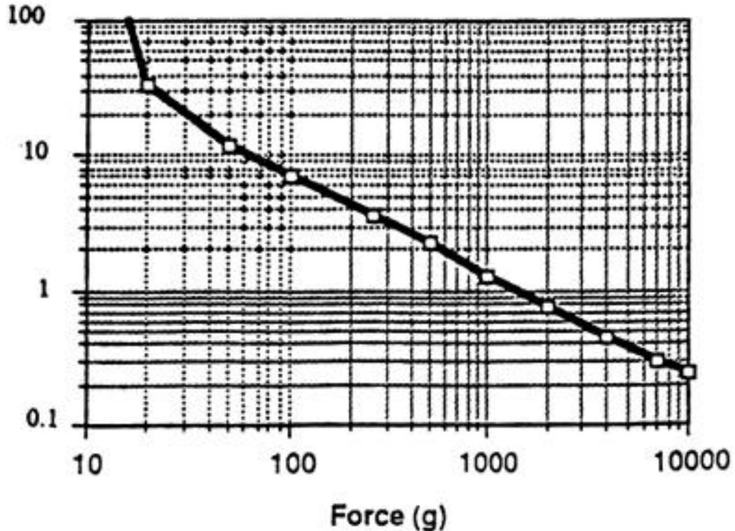
Figure 4. FSR response. The vertical axis represents resistance.<sup>20</sup>
