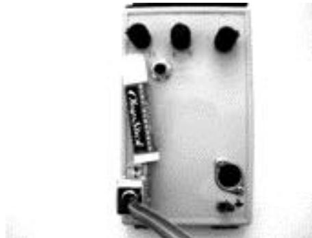
Figure 8. R-Bow belt-mounted computer (with ChapStick for scale)
