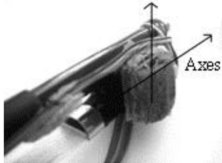
Figure 5. R-Bow frog (with accelerometer axes illustrated)
