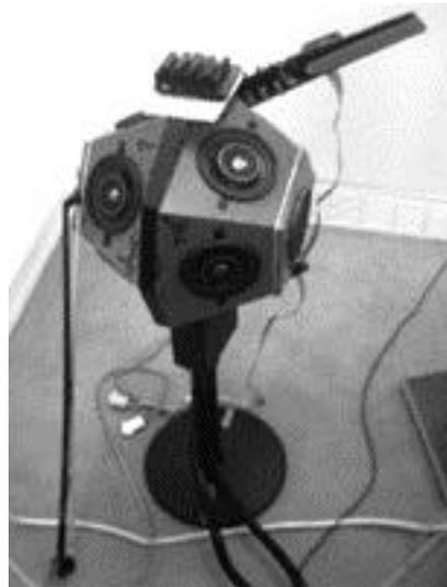
Figure 12. BoSSA (Bowed-Sensor-Speaker-Array)
